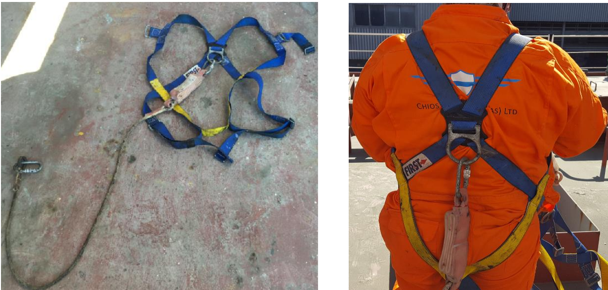
Figure 12: Full body safety Harness used by the Bosun on the morning of the accident
