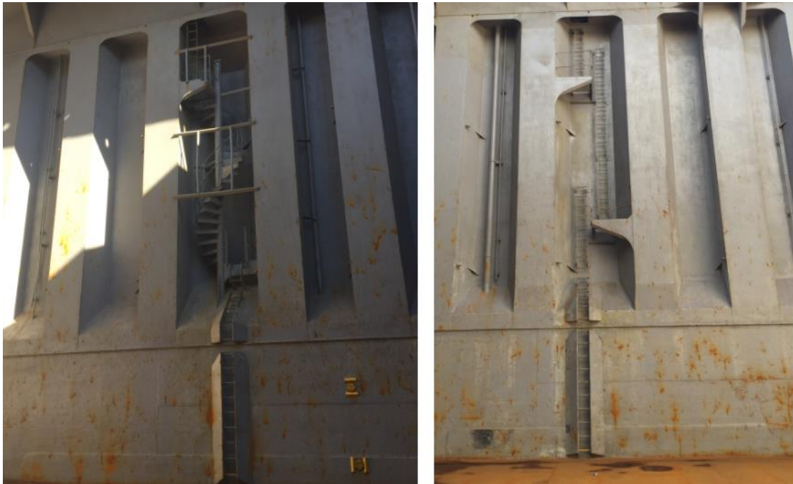
Figure 10: Left: Australian ladder –Right: vertical ladder
