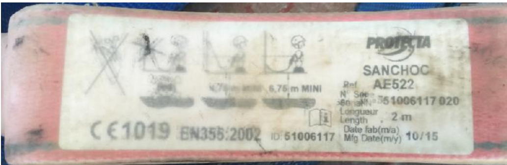
Figure 13: The safety harness label markings used on the day of the marine accident.
