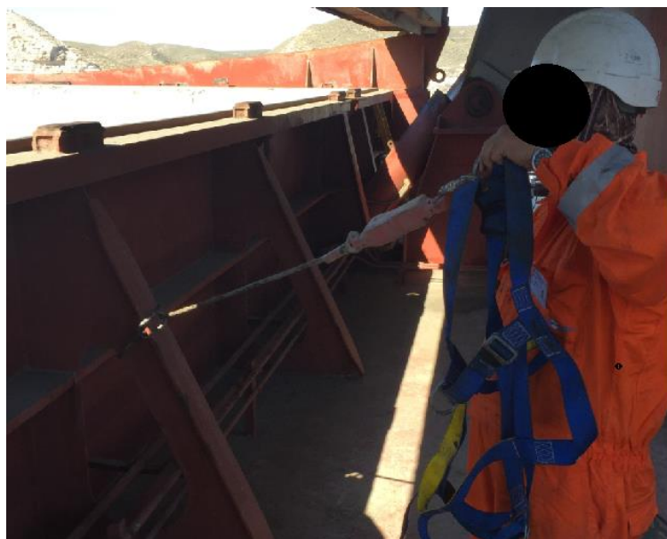
Figure 4 :Simulation by a crew member securing the safety harness on the hatch coaming of cargo hold No.3.
